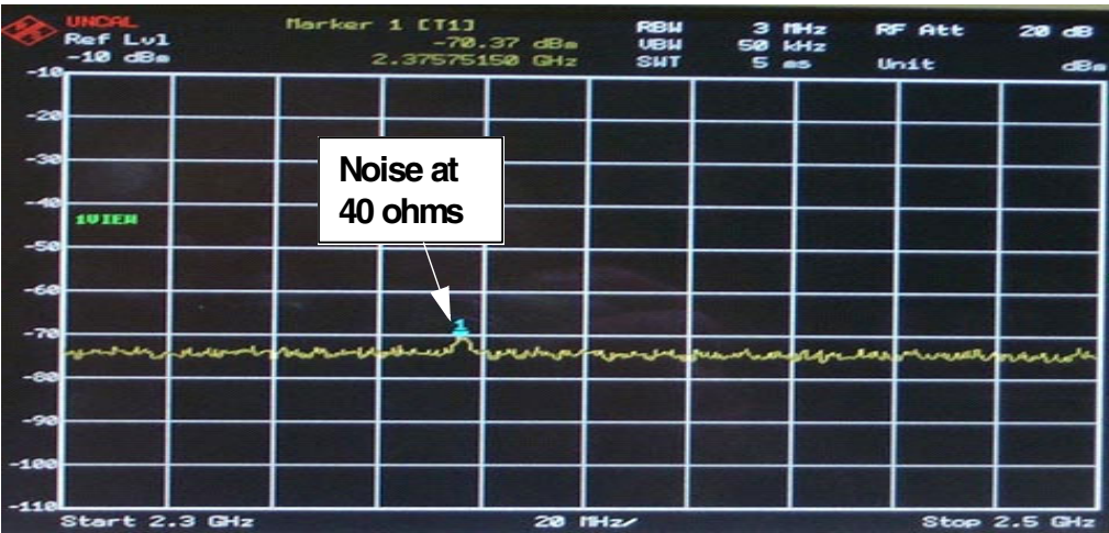
Figure 11. Noise Reduced for 2.3–2.5 GHz with 40-Ohm Memory Clock Driver at 100 MHz Memory Bus Speed
