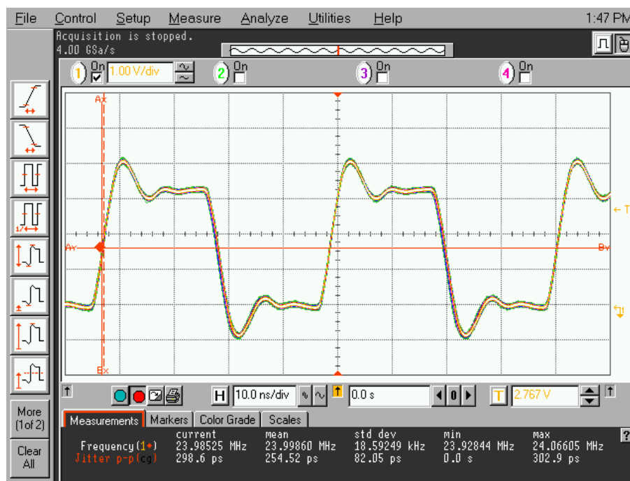
Figure 13. Peak-to-peak jitter of single-ended 24.000 MHz CLK02 (A17 ball) output of SABRE-AI design (i.MX 6Solo, OBDS)
