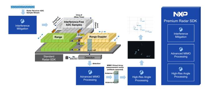
PREMIUM RADAR SDK COMPLEMENTS CUSTOMER RADAR SIGNAL PROCESSING CHAIN
