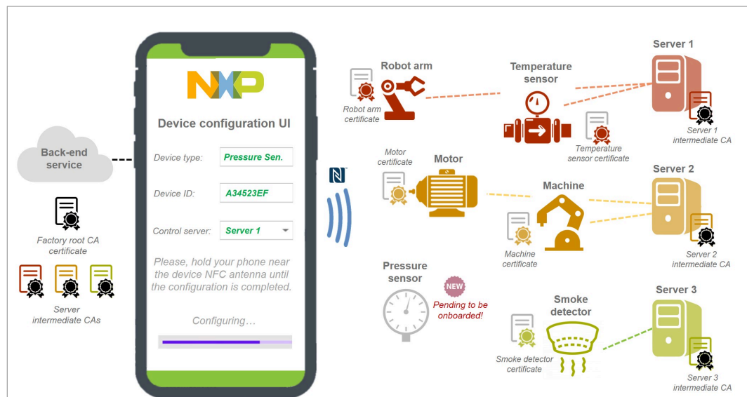
Figure 8. Example of phone application UI for device late-stage credential provisioning
