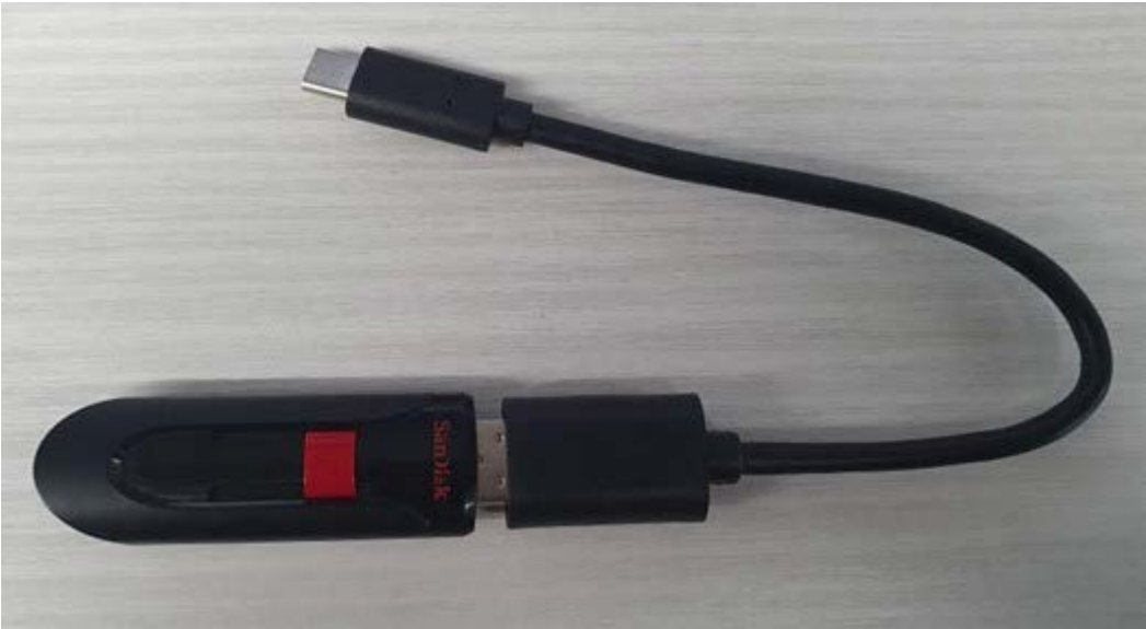
Figure 14. USB-C to USB adapter connections
