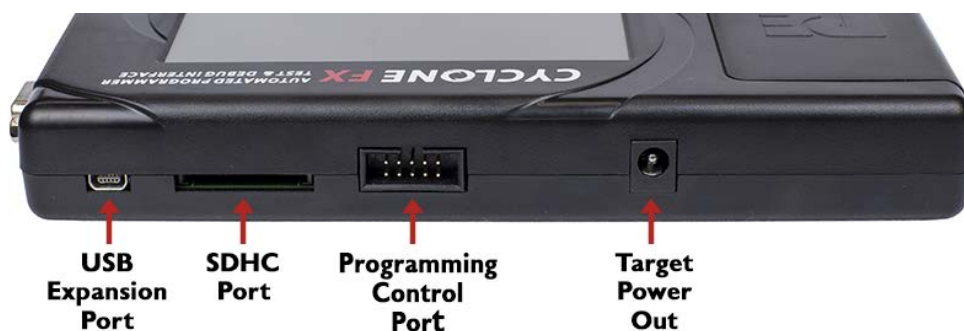
Figure 3-4: Cyclone FX Rear Side View
