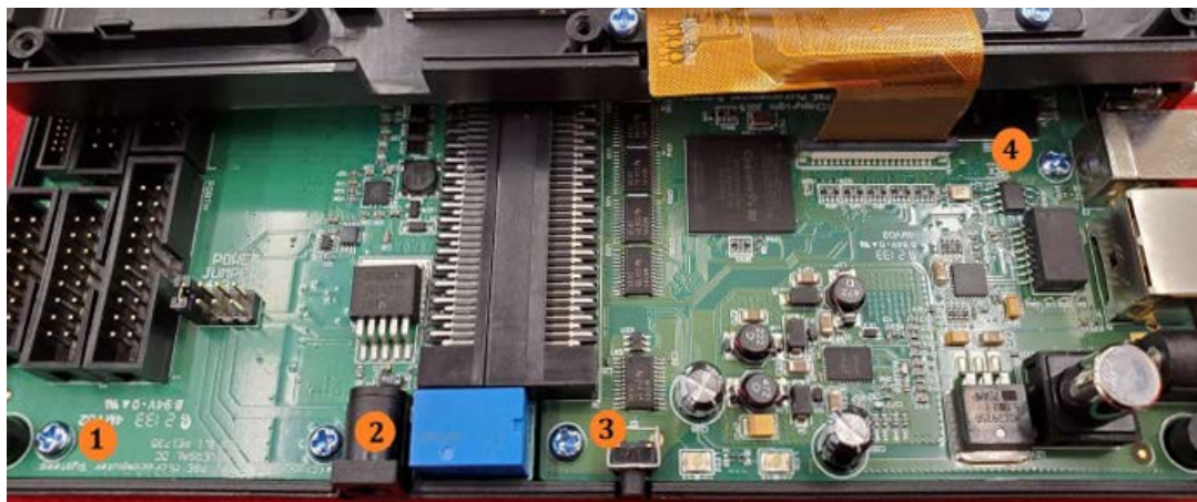
Figure 17-5: Bottom Half of PCB, Four Screws
