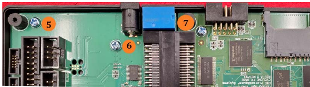
Figure 17-6: Top Half of PCB, Three Screws
