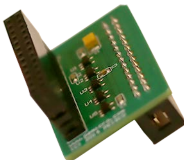
Figure 3-25: ColdFire Adapter (part# CABLE_CF_ADAPTER (Rev. B), for synchronous ColdFire targets, sold separately)
