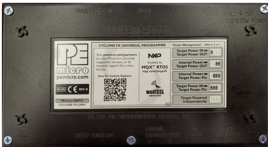
Figure 17-4: Rear Cyclone Case, Five Screws
